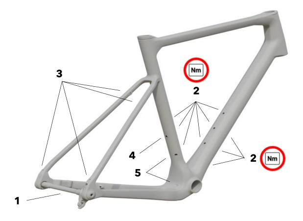
! Maximum torque for bottle cage bolts: 4 Nm
