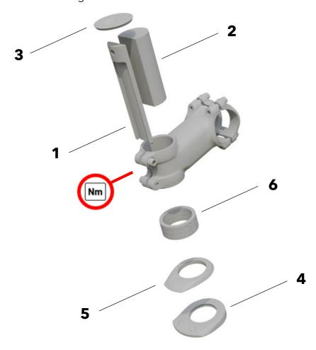
! Maximum torque of cockpit bolts: 6 Nm
