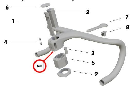
! Maximum torque of cockpit bolts: 6 Nm
